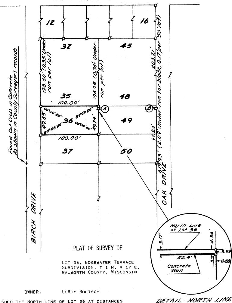
NOTE: ESTABLISHED THE NORTH LINE OF LOT 36 AT DISTANCES CONSISTENT WITH UNDERRUN BETWEEN EXISTING MONUMENTATION. IRON PIPE A AND B ARE NOT CONSISTENT WITH OTHER MONUMENTATION FOUND.
